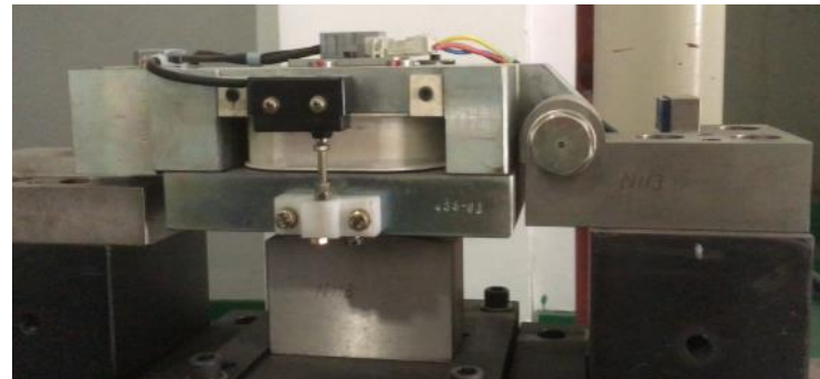
Setting of traction brake static test
