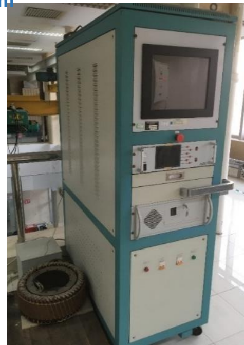
Testing Device of Partial Discharge
