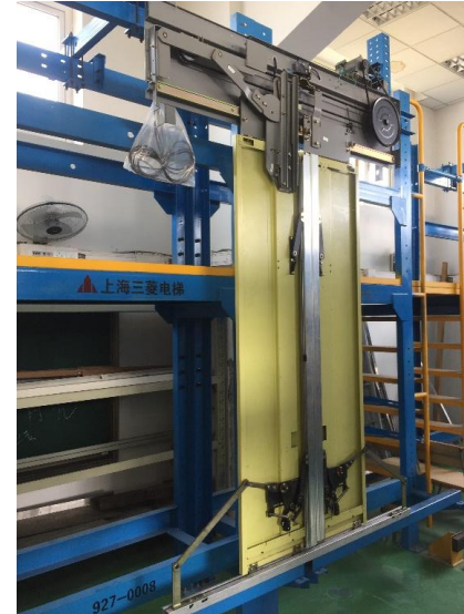
Door machine system testing structure
